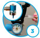
Attach the oxygen tube to the connector or flow meter.
