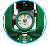
Check the contents gauge to ensure the cylinder is not empty
